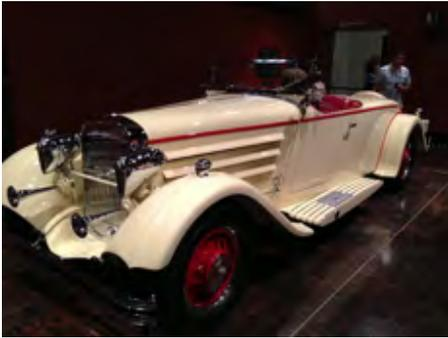
1930 Jordan Model Z Speedway Ace cost \$5,500 in Depression era dollars, with Woodlite headlamps and thermostatically controlled radiator louvers.
