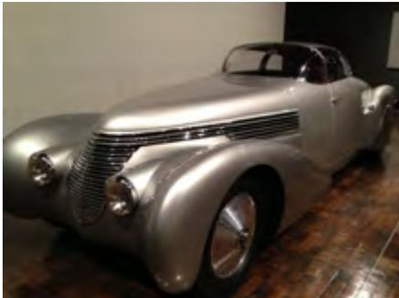
1938 Hispano-Suiza H6B "Xenia" with a curved glass windshield, plexiglass side windows and gullwing doors. It had airline style gauges and a 6.5 liter inline six.
