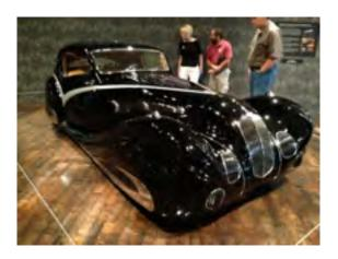
With its sleek aerodynamic styling, the 1936 Delahaye 135M was intended for rally competition. Built on one of 50 short chassis, the body is aluminum, it has a four liter engine, a four speed transmission, and the dash includes a state-of-the-art Jaeger rally clock. The windshield swings out at the bottom for ventilation and the top has a sliding sun roof.
