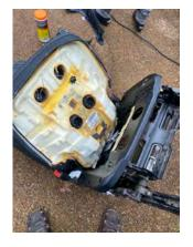
it only required removing the four screws holding the frame to the power seat adjuster, sliding the old cushion out, sliding the new cushion in and re-attaching the four screws. There are a couple of electric connectors to simply unplug before removing the cushion.
